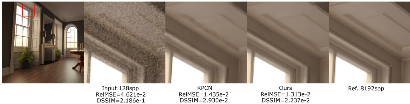
Fig. 1 Comparison of output of our network and the Kernel Predicting Convolutional Network (KPCN) using the same dataset for training. Our model preserves details better, due to the novel network structure, a new feature (light transport covariance in path space), and the perceptual loss function. Quantitative error metrics (RelMSE and DSSIM) also confirm the higher quality of our method.
