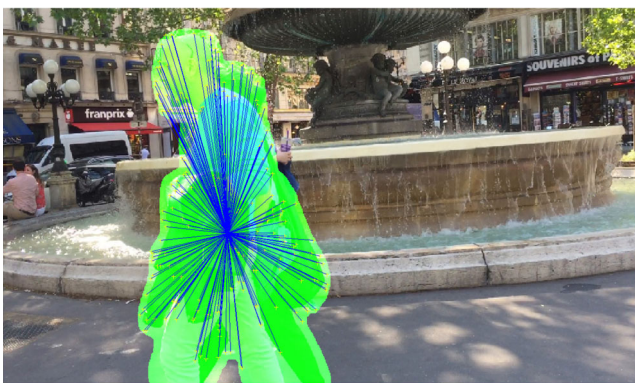
Fig. 5 Region description. Each region is described by a global histogram, a set of SURF keypoints (yellow points), and a set of vectors which connects each keypoint and the centroid of the region.
