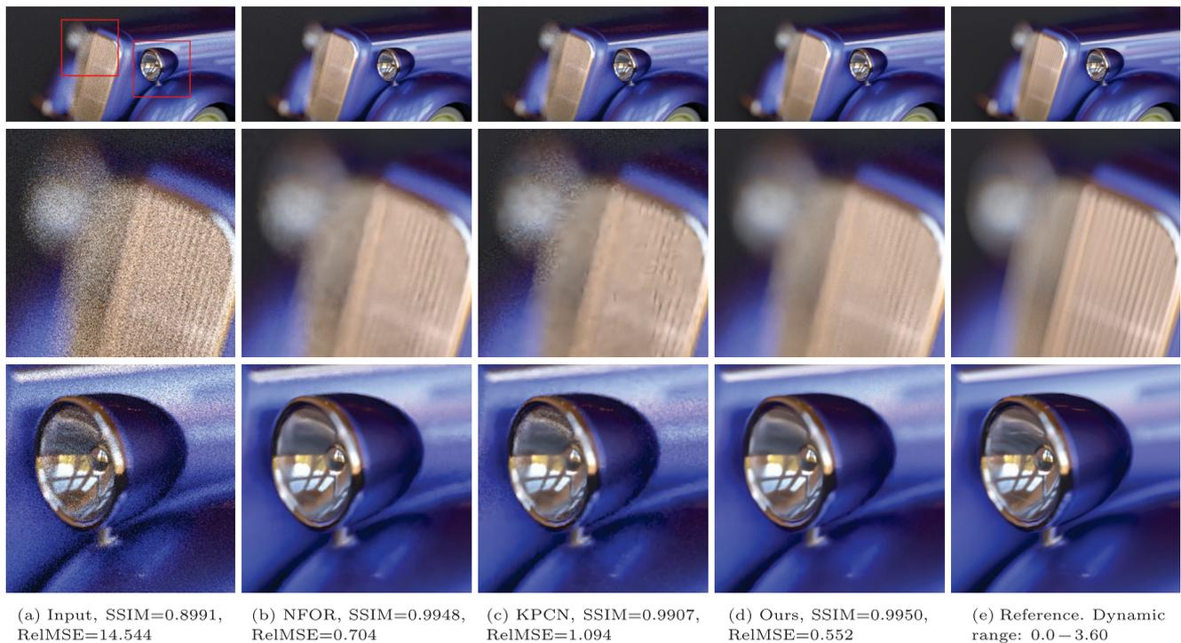
**Fig. 12** Car scene. Input (32 spp) and reference (8192 spp) images rendered by Tungsten. Quality metrics refer to the top row images. RelMSE ( $10^{-3}$ ).
