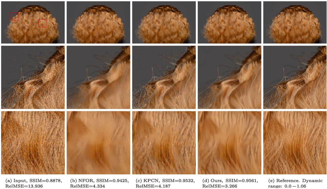
**Fig. 13** Hair scene. Input (32 spp) and reference (2048 spp) images rendered by Tungsten. Quality metrics refer to the top row images. RelMSE ( $10^{-3}$ ).
