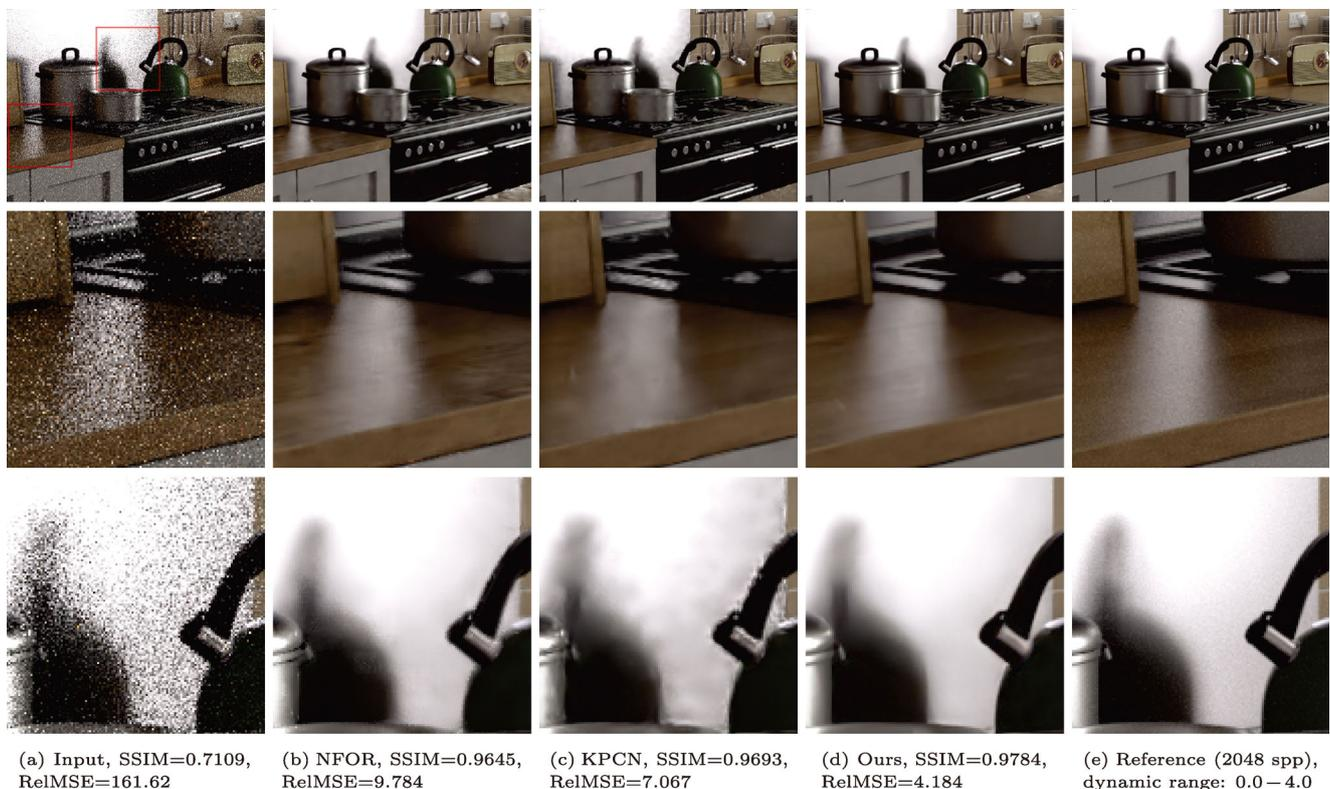
**Fig. 10** Kitchen (close-up). Input (16 spp) and reference (2048 spp) images rendered by Tungsten. Quality metrics refer to the top row of images. RelMSE ( $10^{-3}$ ).
