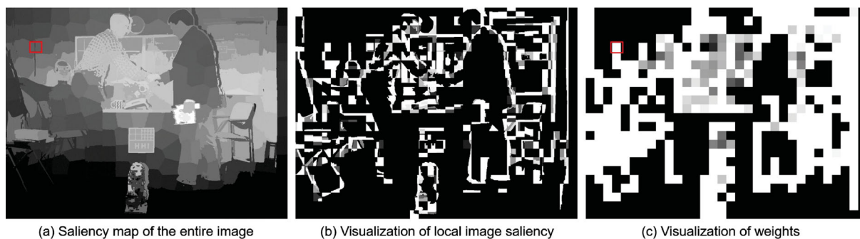
Fig. 8 Visualization of local image saliency based weighting. (a) Saliency map of the entire distorted image. (b) Merged saliency maps of the associated small image patches. All saliency maps were produced by Ref. [28]. (c) Local image saliency based weights, brighter blocks indicating higher weights.
