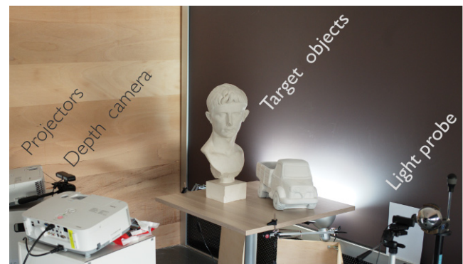
Fig. 2 An example setup with two projectors, a depth camera for tracking, and a diffuse white target object.
