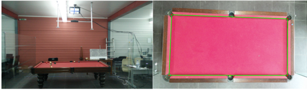
Fig. 1 Left: prototype. Right: a region of the colour frame acquired by the Kinect, with the 4 corners (and rails) marked.
