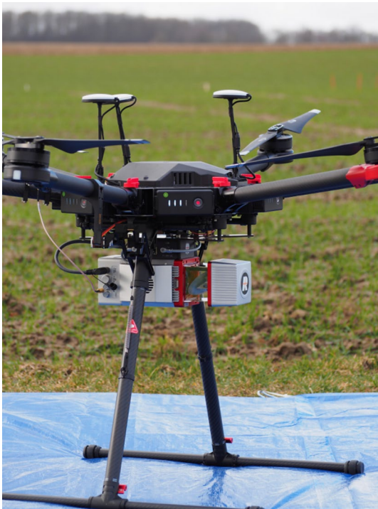
Fig. 2 The system used in this study, which is a UAV DJI Matrice 600 pro, with a Riegl Mini-VUX-1 LiDAR scanner
