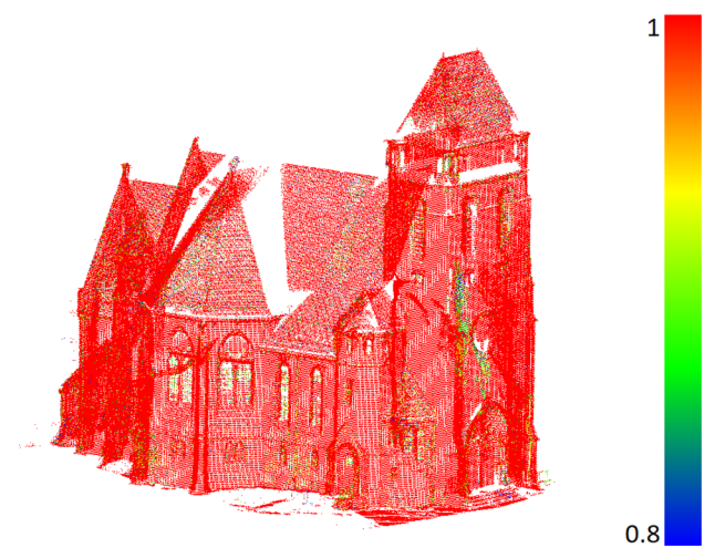
Fig. 11 Example voxel grid of the “Lutherkirche”, coloured by W_{static} from 0.8 to 1 (the tree from Fig. 9 was cut out to show the complete facade)
