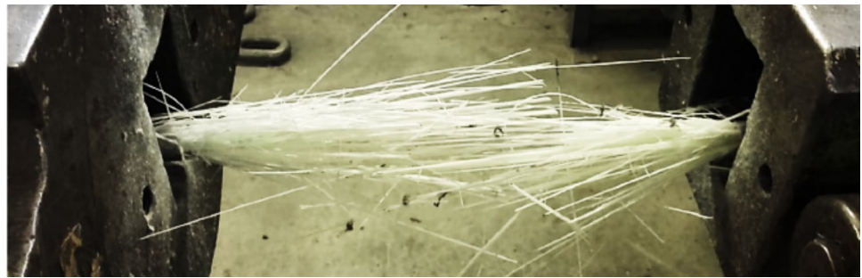
Fig. 4 Failure of an FRP rebar under tension, Antino et al. [36]
