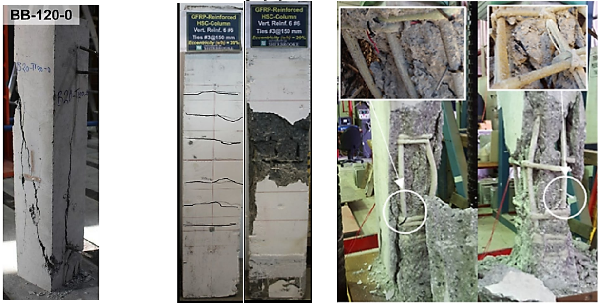
(b) Concrete crushing at mid-height [47]
