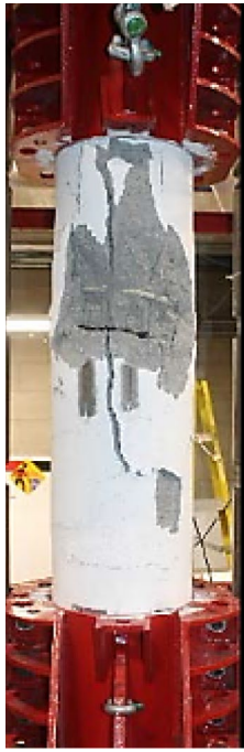
(a) Vertical crack on the compression side [44]
