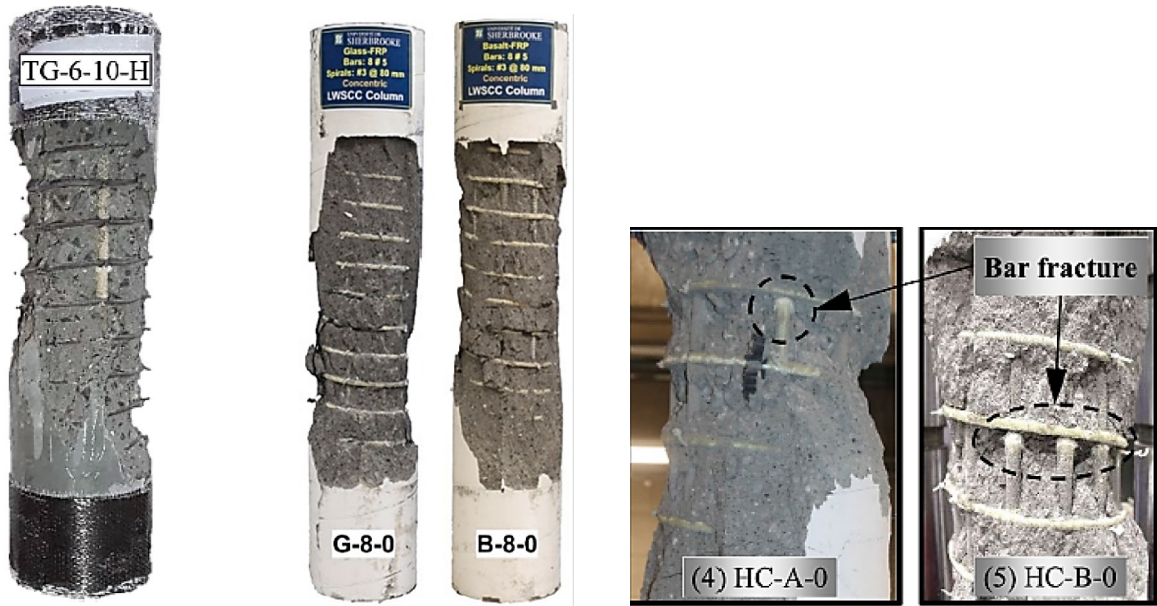
(b) Concrete crushing at mid-height [47]
