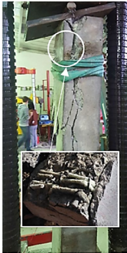
(d) Slipping of GFRP rebars near the top [53]
