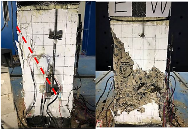
(g) Crack distribution at mid-height of column [49]
