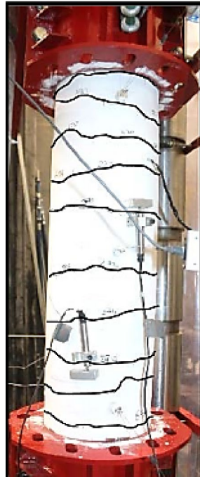
(b) Horizontal cracks on the tension side [44]
