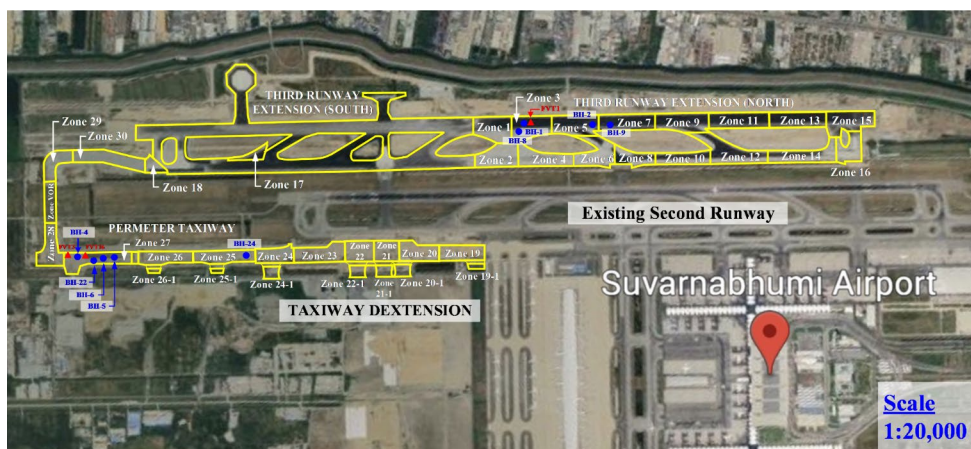
Fig. 2 Locations of zones 5 and 7 and zones 25 and 27 and corresponding bore holes in the third runway extension (North) and taxiway D extension, respectively
