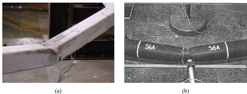
Fig. 7 Experimental deformed configuration: a HSS section, and b HCS section
