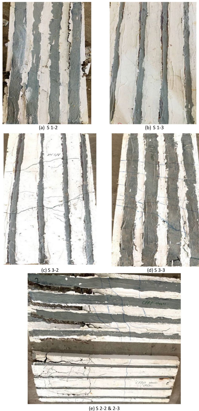
Fig. 8 Failure Crack Modes for Tested slabs; a) and b) group 1, c) and (d) group 3, and e) group 2
