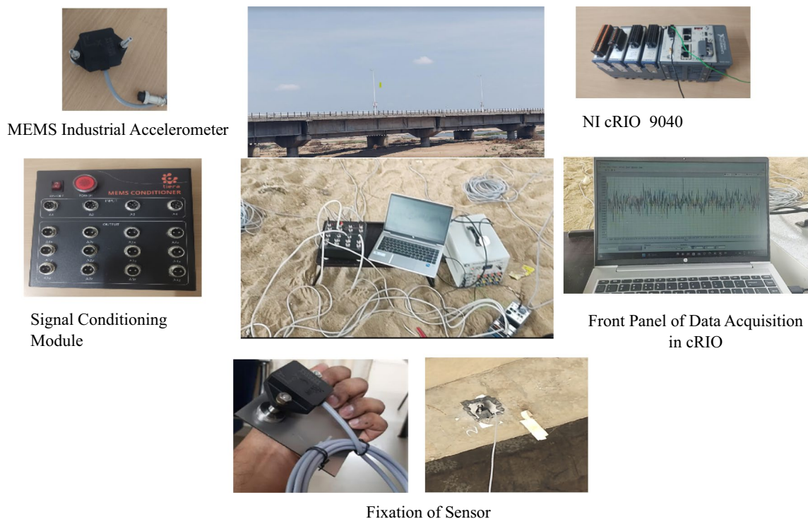
Fig. 15 Field Test: Data Acquisition from the bridge
