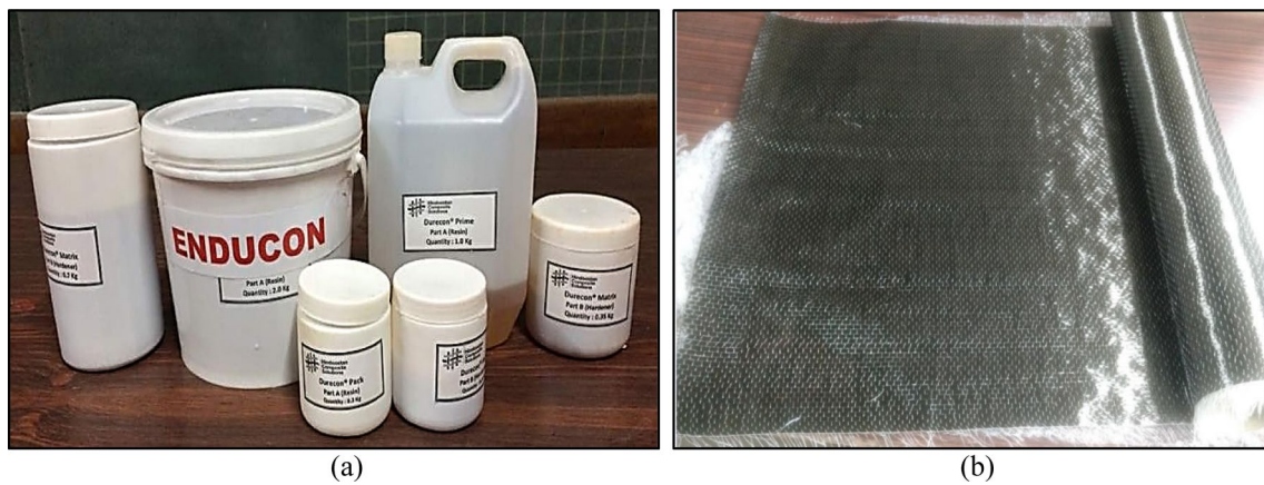
Fig. 2 Strengthening materials, (a) Resin and hardener, (b) CFRP Sheet
