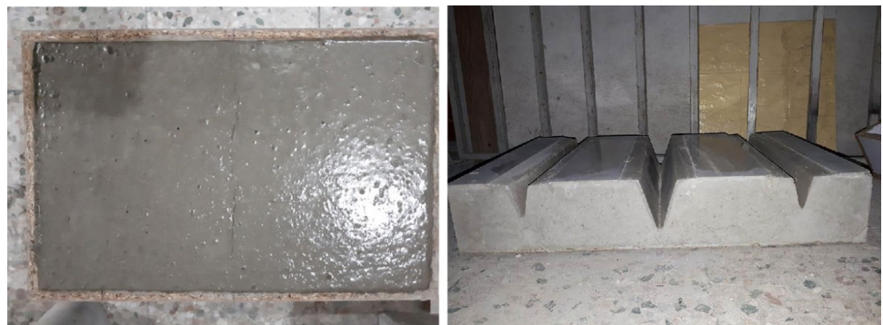
Fig. 4 the cracked sample under plastic shrinkage conditions
