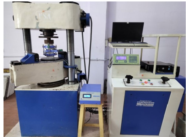
Fig. 7 Modulus of elasticity test setup
