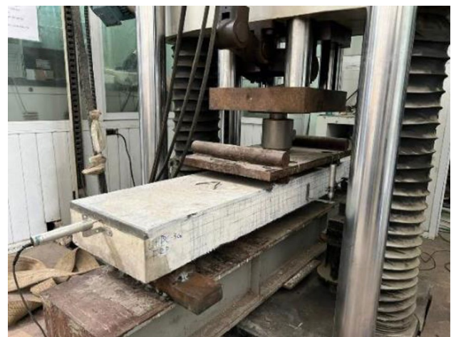
Fig. 4 Point of view of four-point bending test
