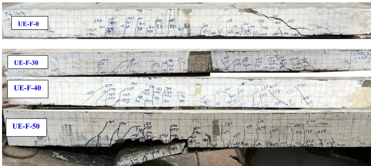
Fig. 10 Modes of failure and crack patterns of UE-F series
