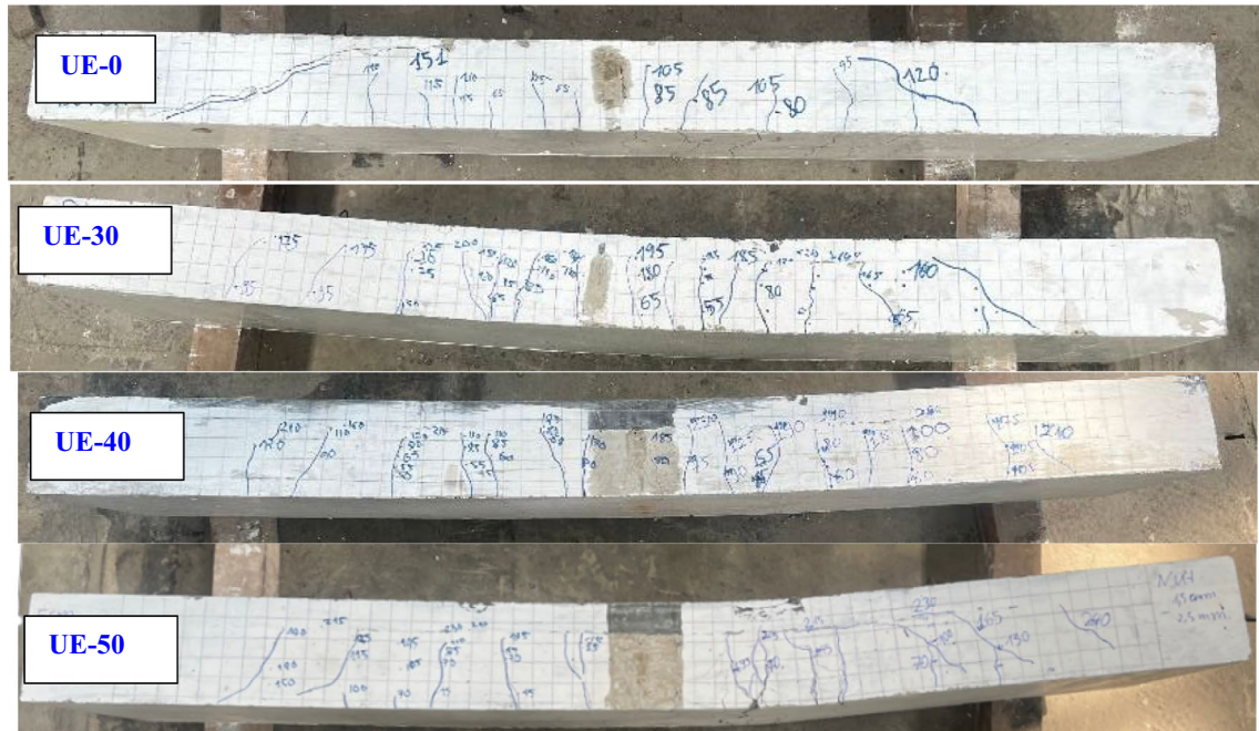
Fig. 8 Modes of failure and development of crack observed in the UE series
