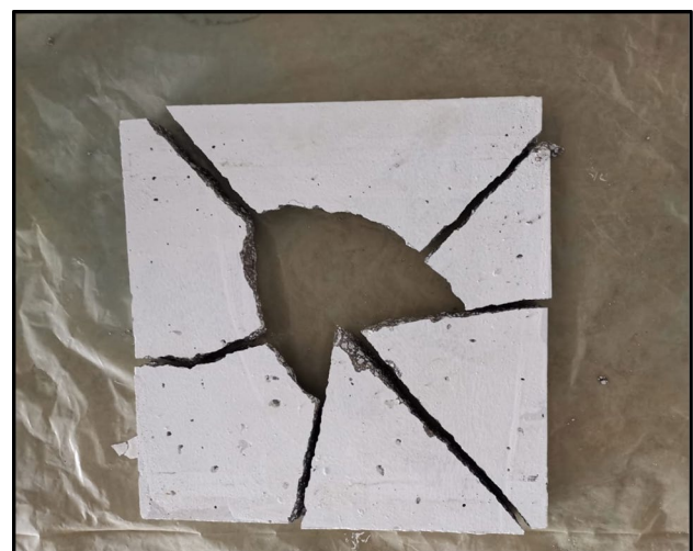
Fig. 29 Failure Pattern of control specimen
