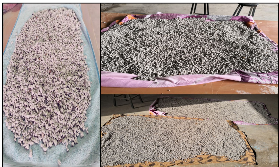
Fig. 4 spread out the light-weight aggregates to have SSD condition
