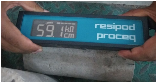
Fig. 8 Surface resistivity measurement
