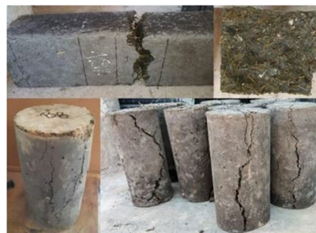
Fig. 8 Cylindrical and prismatic specimens of geopolymers tested. Source: Authors
