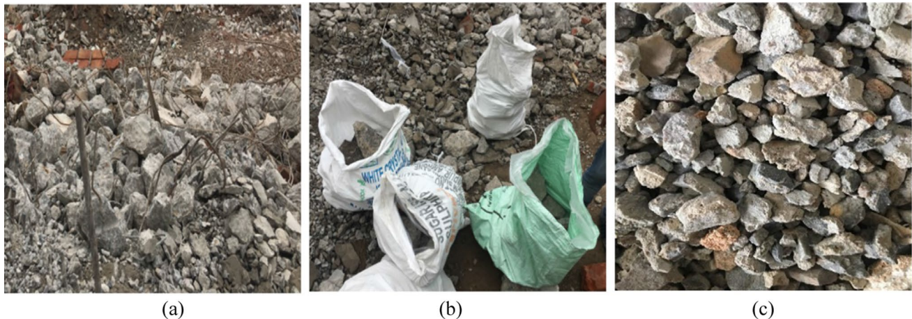
Fig. 2 Generation of recycled coarse aggregate: a demolished concrete blocks; b transportation of concrete blocks in plastic bags; and c RCA prepared in the laboratory
