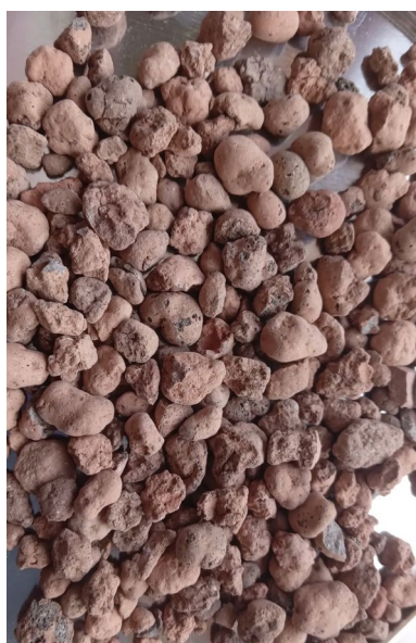
Fig. 2 Expanded clay LACA used as coarse aggregate
