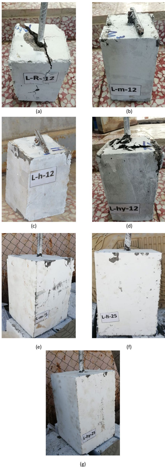
Fig. 11 Failure modes of the lightweight concrete mixes; a L-R; b L-M-12; c L-H-12; d L-HY-12; e L-M-25; f L-H-25; g L-HY-25
