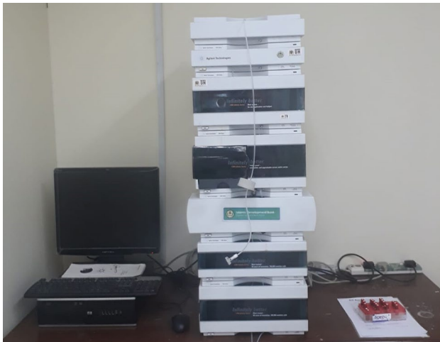
Fig. 2 GPC experimental setup Agilent 1260 Infinity Quaternary LC equipment
