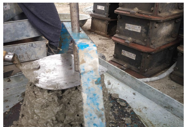
Fig. 7 Slump value of reference mix
