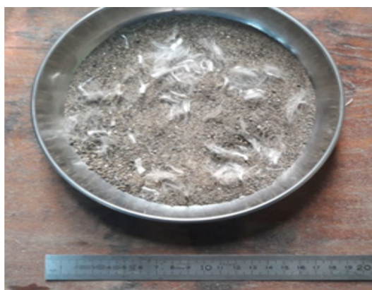
Fig. 4 Chlef sand mixed with polypropylene fibers (Sika)
