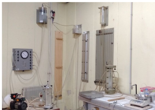
Fig. 3 Permeability apparatus used in this study
