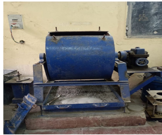
Fig. 10 Cantabro test using LAA Machine
