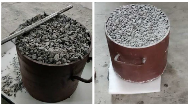
Fig. 3 Bulk density mould with open graded sample
