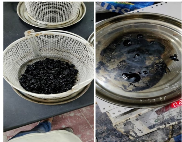
Fig. 5 Drain down loss before and after testing
