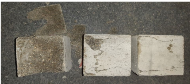
Fig. 7 Failure of conventional mortar cubes
