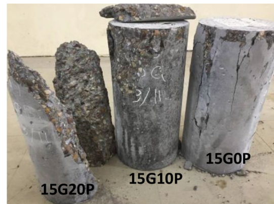
Fig. 14 Failure shape of cylindrical samples under compressive load
