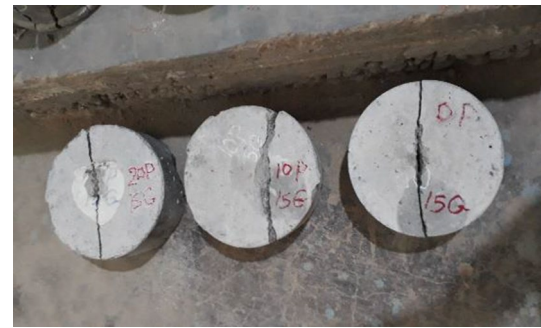
Fig. 21 Specimens failure shape under impact load
