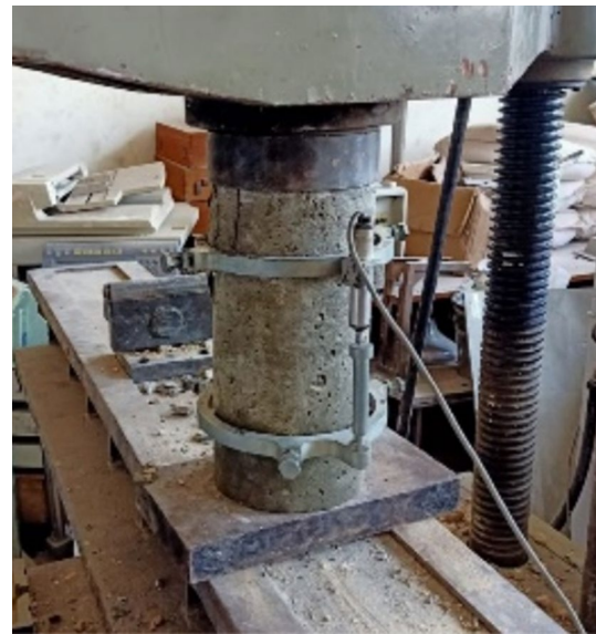
Fig. 3 Static modulus of elasticity and Poisson’s ratio determination test
