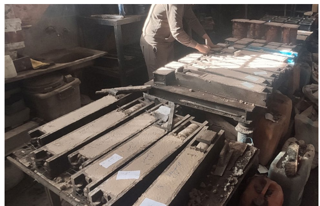
Fig. 1 Specimens of compression strength, flexure strength, modulus of elasticity and Poisson's ratio tests
