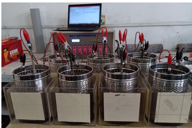
Fig. 4 Accelerated corrosion test setup
