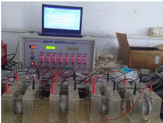
Fig. 3 Rapid chloride permeability test setup
