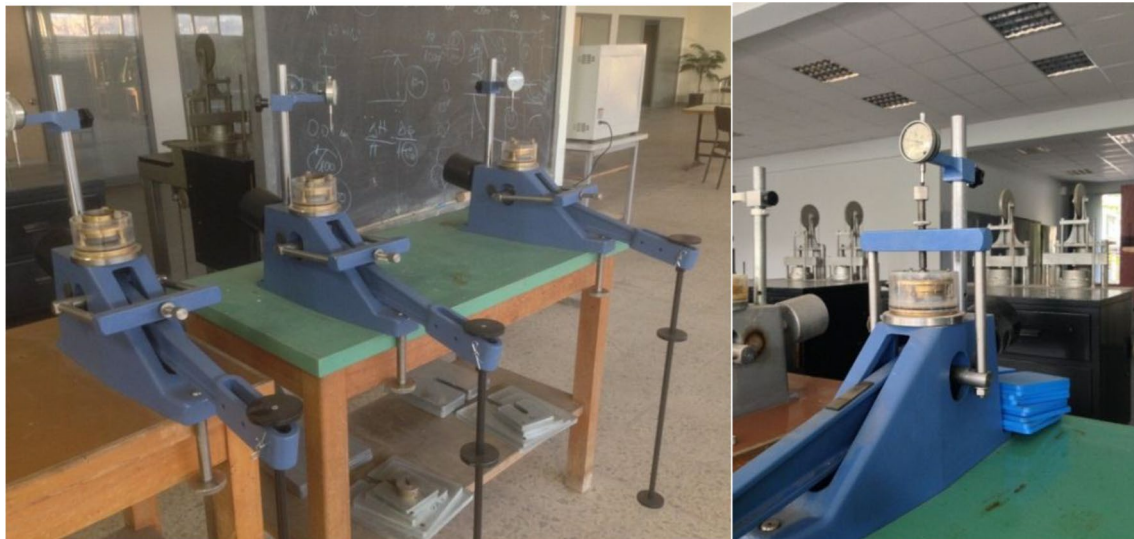
Fig. 7 Experimental setup (oedometer apparatus)
