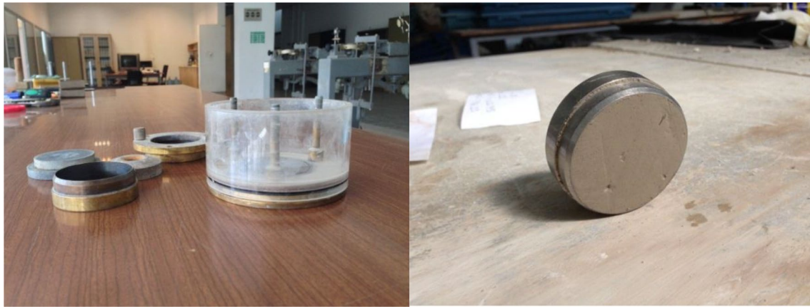
Fig. 8 Consolidometer cell equipment (the left image) and a compacted soil sample in the ring (the right image)
