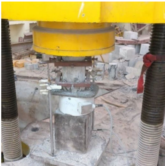
Fig. 1 LVDT’s setup attached to the cylinder
