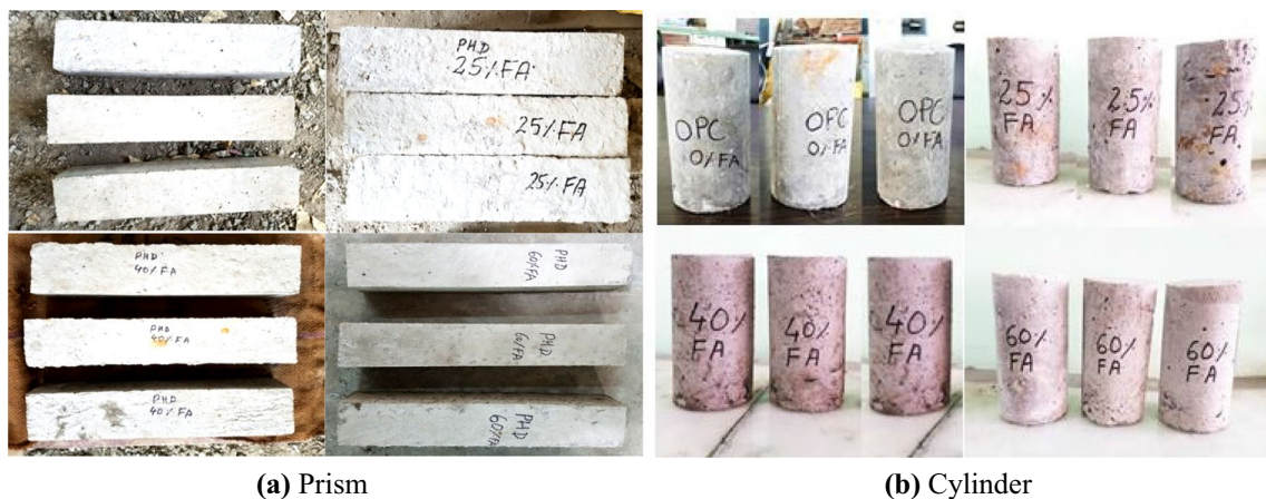
Fig. 3 Concrete specimens for flexural and splitting tensile strength of concrete
