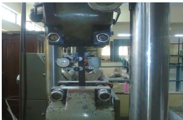
Fig. 3 Steel tube coupon test
