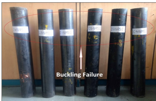
Fig. 8 Experimental failure modes under compression
