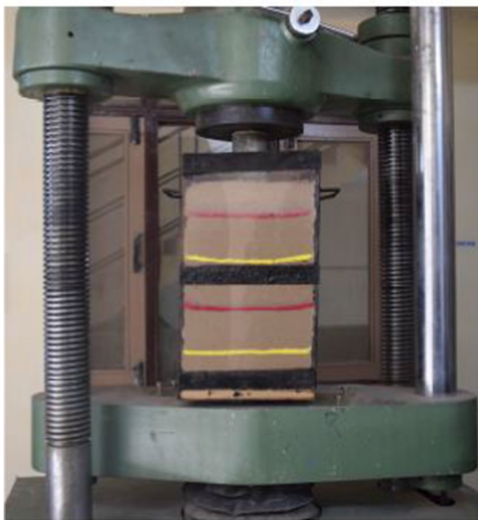
Fig. 9 Testing of stone columns set up under UTM
