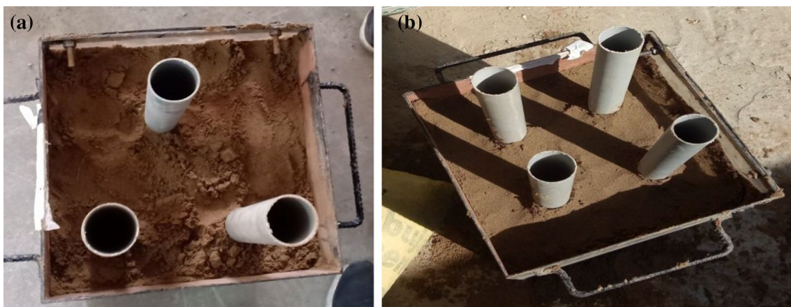
Fig. 5 a Unreinforced group of 3 stone columns. b Unreinforced group of 4 stone columns
