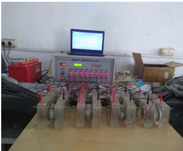
Fig. 4 Experimental setup of rapid chloride permeability test
