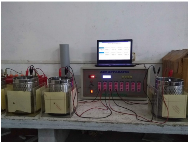
Fig. 5 Experimental setup of accelerated corrosion test
