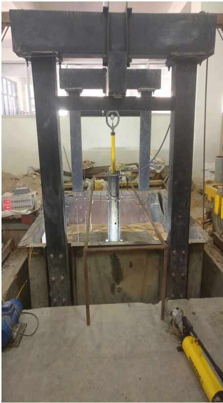
Fig. 6 Experimental setup for repeated load test
