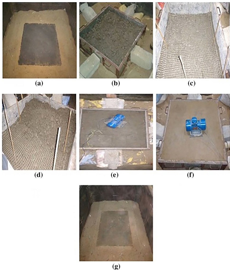
Fig. 3 Pictorial view of construction of model pavement section. a compacted subgrade, b partially compacted GSB, c geogrid with sakes, d geogrid layer with overlying GSB material, e compacted GSB, f compacted sacrificial layer, g model pavement section surrounded by sand
