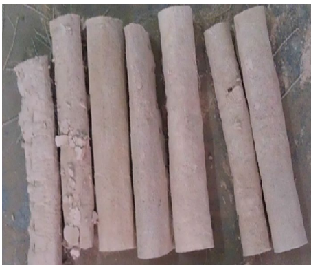
Fig. 13 Geosynthetic-encased stone columns
