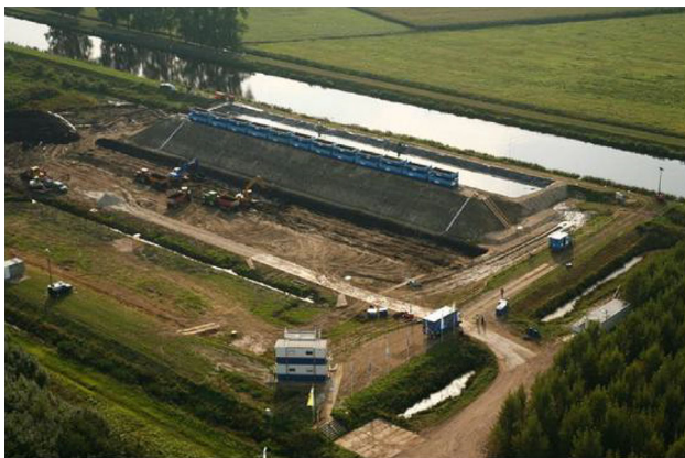
Fig. 3 Aerial view of the stability test levee [5]
