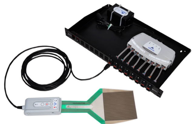
Fig. 7 Tactile pressure sensor connected to the handle and to the tactile DAQ computer [8]
