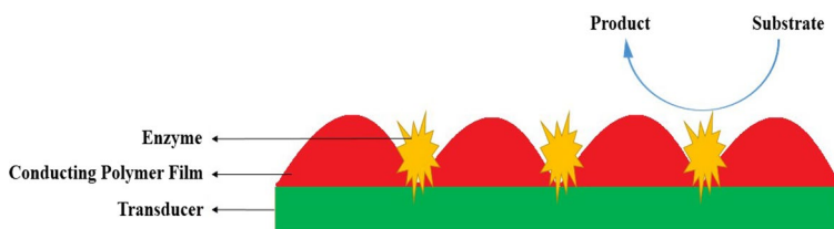
Fig. 15 Schematic representation of a bio-sensing system
