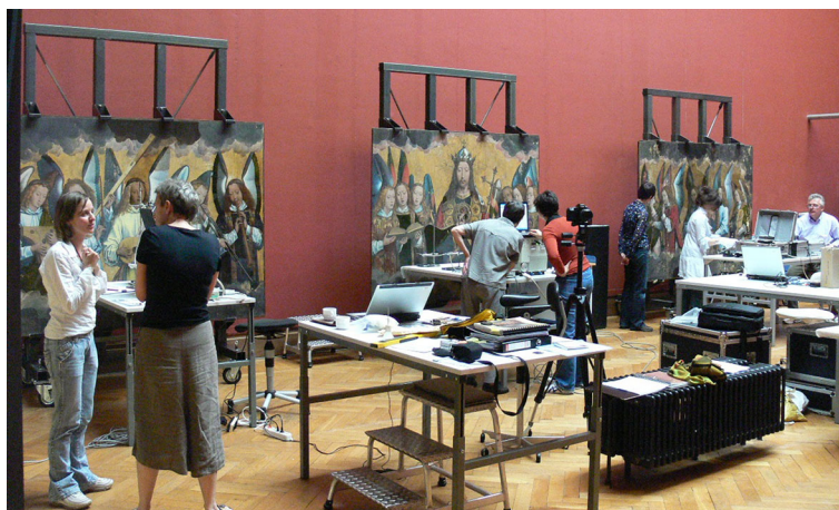
Fig. 1 The mobile laboratory, MOLAB, during the campaign at the Royal Fine Art Museum of Antwerp for the study of the triptych Christ among Singing and Music Playing Angels (ca. 1487–90), by H. Memling. The analytical work is proceeding simultaneously applying different techniques. The instruments rotate in front of each panel in order to investigate the selected areas with all the available equipment
