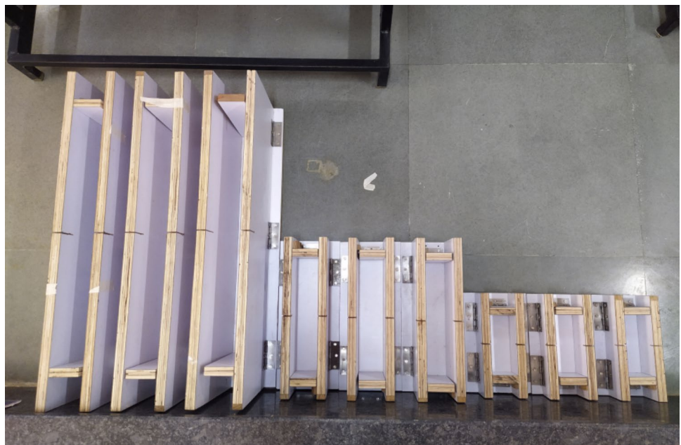
Fig. 2 Molds of specimens for concrete
