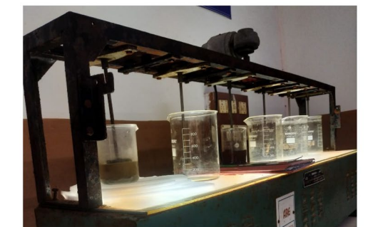
(c) Jar-test apparatus for making solution for titration
