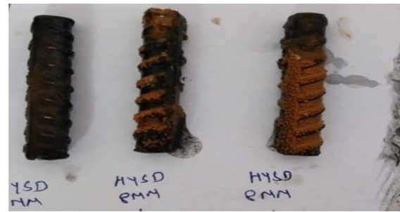
(b) CS bars after 28 days of immersion
