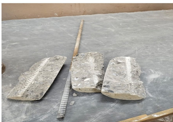
(a) Bond failure Before Corrosion
