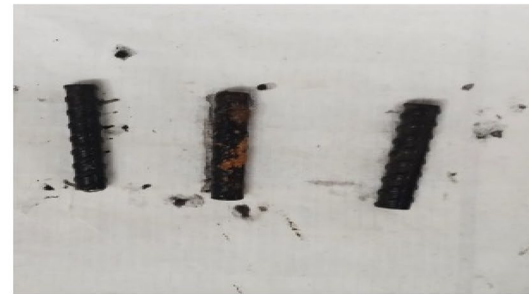
(b) CS bars after 28 days of immersion
