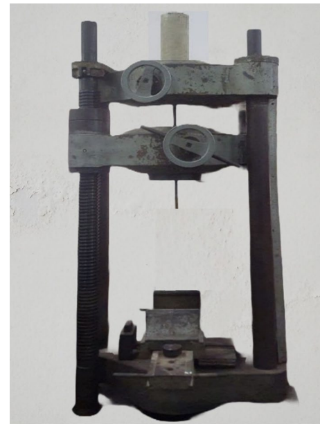
Fig. 5 Bond test for CS and SS specimens
