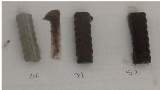
(a) SS bars after 28 days of immersion
