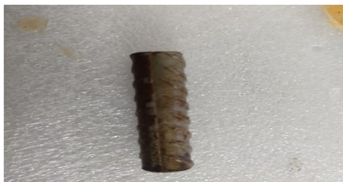
(e) SS 8mm bar after 365 days of immersion in 5% NaCl medium
