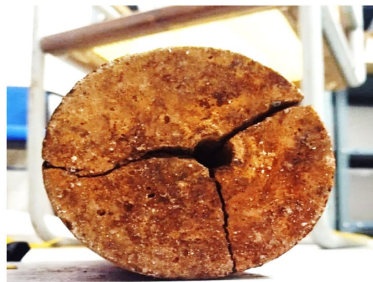
(b) Bond failure after Corrosion
