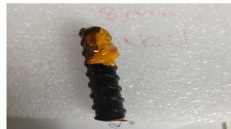
(f) CS 8mm bar after 365 days of immersion in 5% NaCl medium
