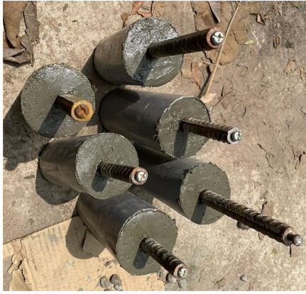
Fig. 2 Cylinder specimens for ACT and pull-out test
