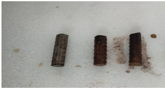
(a) SS bars after 28 days of immersion
