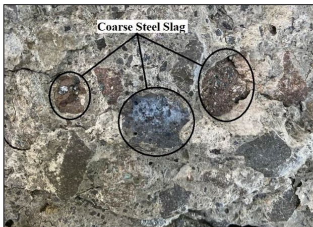
Fig. 15 CSSA bonding in concrete
