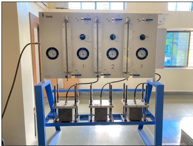
Fig. 9 Water penetration test (setup)
