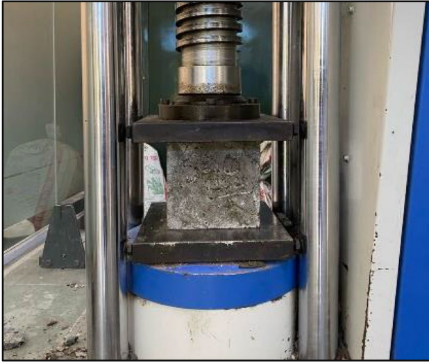
Fig. 6 CS test of concrete on cube sample ( 150 \times 150 \times 150 mm)
