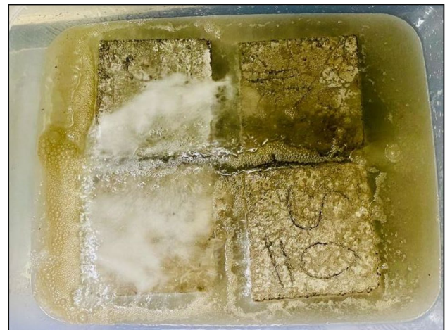
Fig. 11 10% conc. HCl (acid attack test setup)
