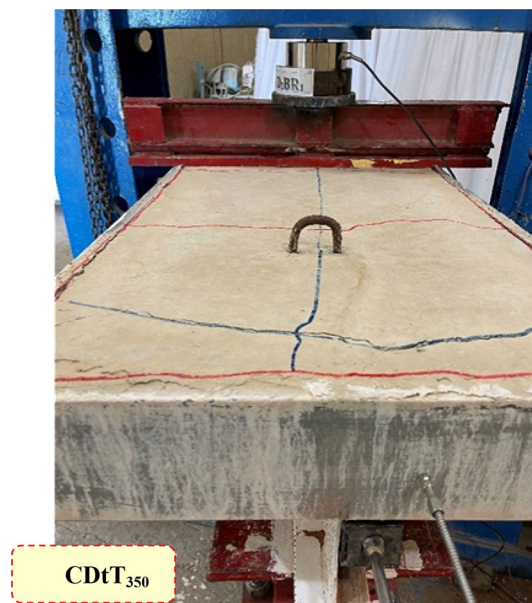
Fig. 23 Thermal and longitudinal cracking in specimen CD2T350
