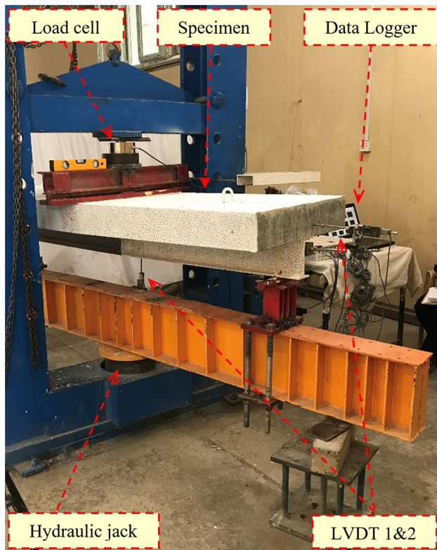
Fig. 10 Description of the testing machine utilized in this study
