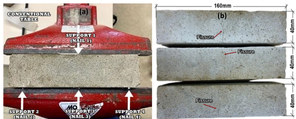
Fig. 2 Opening of cracks in prismatic specimens by means of manual loading in a 4-point bench vice a protocol used b resulting cracks
