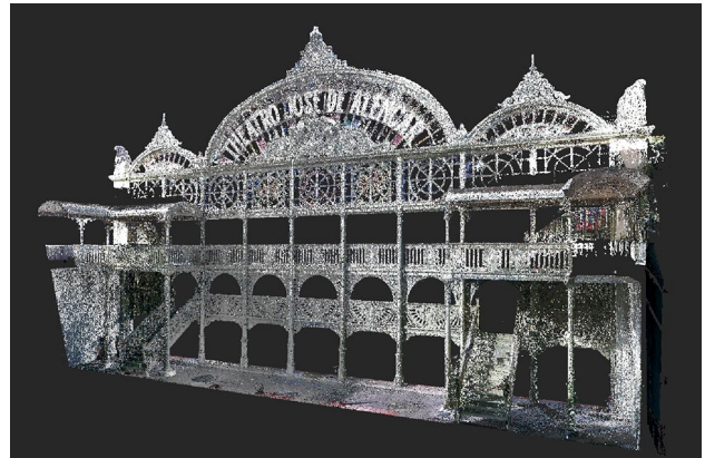
Fig. 10 View of the point cloud after processing in the Recap pro software
