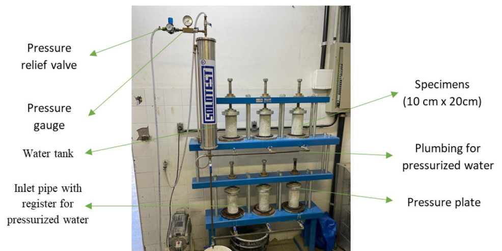
Fig. 2 Pressure water penetration test
