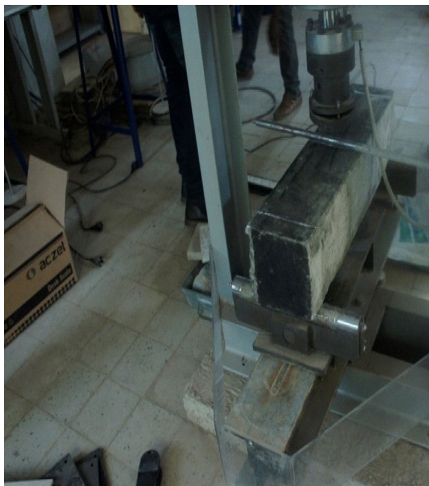
Fig. 8 Flexural strength testing
