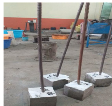
Fig. 2 Samples prepared for the pull-out test
